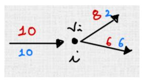
$$\overbrace{8+6}^{\text{uscenti}} - \overbrace{10}^{\text{entranti}} = 4 \text{, } v_i = 4, v_i > 0 \text{, nodo origine} | \\ \underbrace{2+6}_{\text{entranti}} - \overbrace{10}^{\text{entranti}} = -2 \text{, } v_i = -2, v_i < 0 \text{, nodo destinazione}$$
